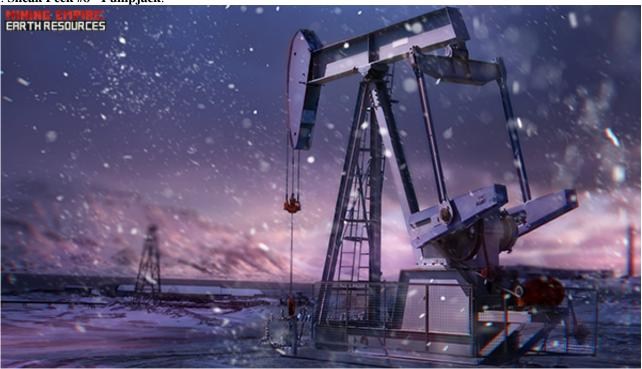
A pumpjack is the overground drive for a reciprocating piston pump in an oil well. It's used in the oil-producing industry to drill wells up to 4,000 meters deep.
